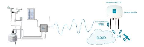
METEO MOTE is able to monitor temperature, relative Humidity, atmospheric pressure, rainfall and dew point (frost).
