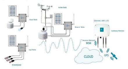
HYDRA MOTE, is the integrated system of irrigation and fertiirrigation, consisting of transceiver boards to be able to define read, control and modulate the parameters coming from the environment.
